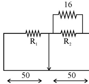
$$\text{here } R_1 = \frac{16R_2}{16+R_2} \dots (2)$$
