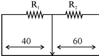
$$\text{here } \frac{R_1}{40} = \frac{R_2}{60} \Rightarrow \frac{R_1}{R_2} = \frac{2}{3} \dots (1)$$
