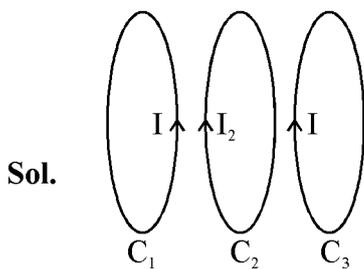
For  $I_2$  to be clockwise $\Rightarrow C_1$  should move towards  $C_2$  so that induced current in  $C_2$  repel  $C_1$ . $\Rightarrow C_3$  should move away from  $C_2$  so that induced current in  $C_2$  attract  $C_3$ .
