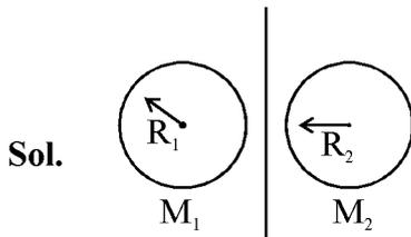
$$I = \left[ \frac{2}{5} M_1 R_1^2 + M_1 R_1^2 \right] + \left[ \frac{2}{5} M_2 R_2^2 + M_2 R_2^2 \right]$$
